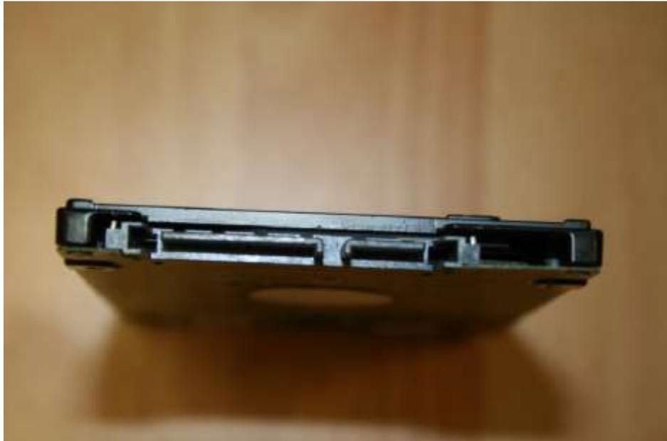
Step 12: Connect the new hard drive to the motherboard and reconnect the wires to other components. Note that the assembly needs to be the same as before the repair.
