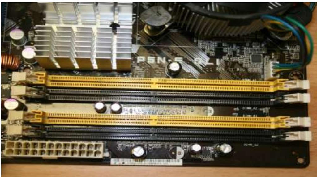
Step 4: Connect the new RAM to the motherboard and connect the clamps on each side making sure they click and lock in place.
